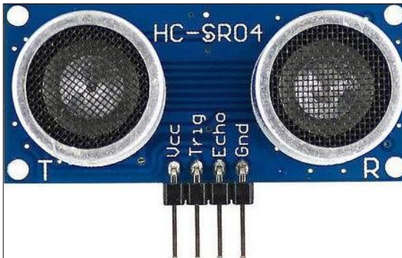
Fig 3: Diagrammatic Representation of ultrasonic sensor [ELECTRONIC HUB]
